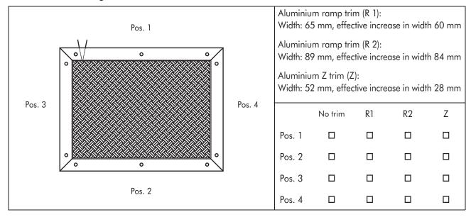
If not stated otherwise, fixing holes are dimensioned by us and their number is determined corresponding to the dimensions. Fixing material (screws, dowels, plugs) is supplied with the mat.
